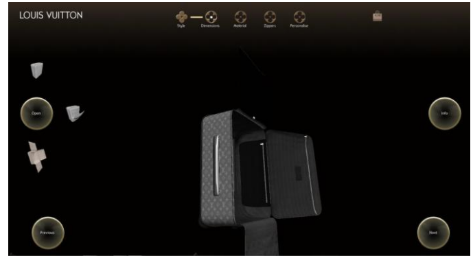
Fig. 5. 3D Product isolation mode. Direct manipulation of the product can be accomplished directly by placing the mouse cursor over the 3D model of the product. GUI elements on the left hand side of the screen under the Open button provided to investigate inside the bag and the inner parts of the compartments if applicable.
