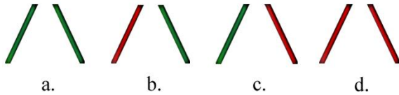
Figure 2. Colour coding of the lane symbols. Key: (a) no obstacles on either side of the vehicle (b) obstructed left side (c) obstructed right side (d) obstacles on both sides of the vehicle
