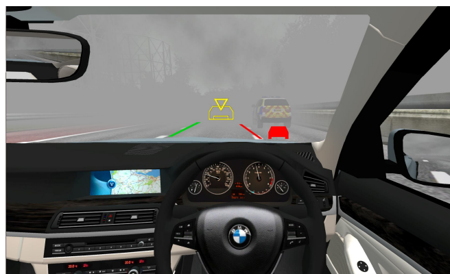
Figure 2: Screenshot of the actual VR Drivign Simulator with enabled HUD interface.
