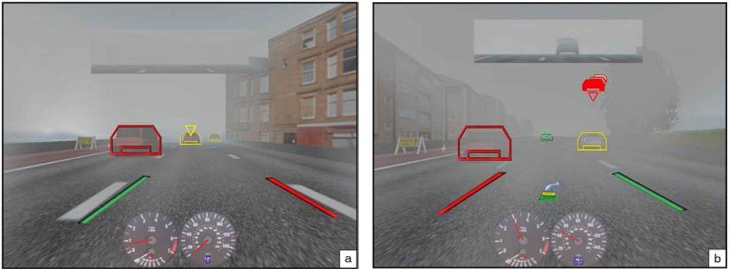
Figure 1: (a) Typical HUD interface configuration, (b) all-symbols configuration
