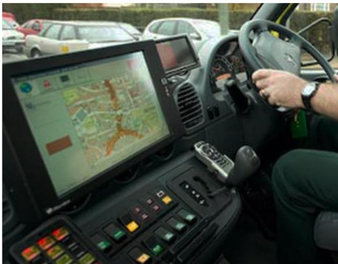
Fig. 2. ES vehicle cabin offering multiple information-provision conduits.
