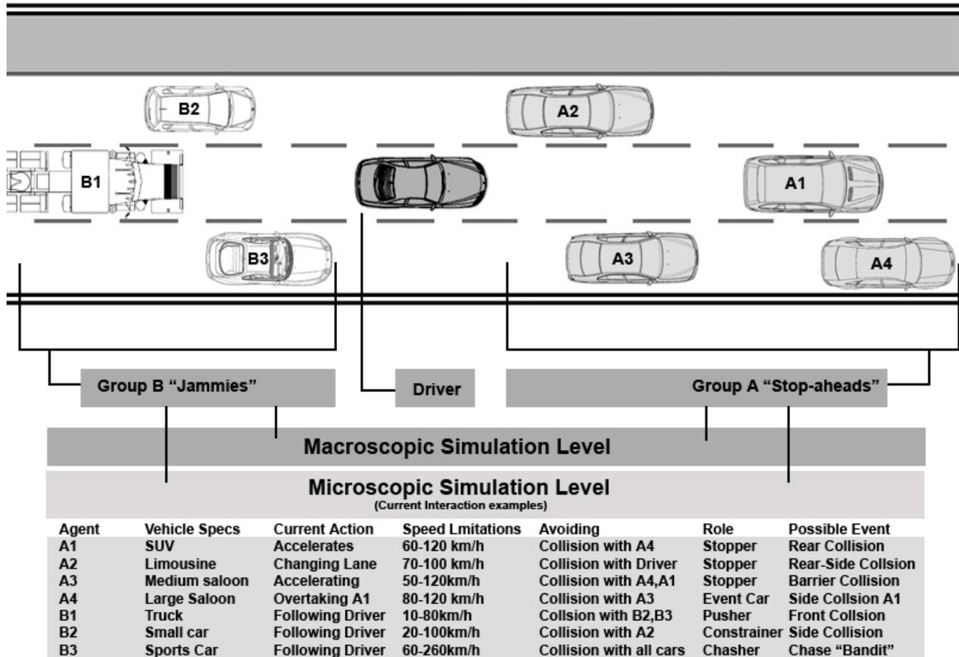
Figure 2. A diagram of the main robot vehicle categories and their functions
