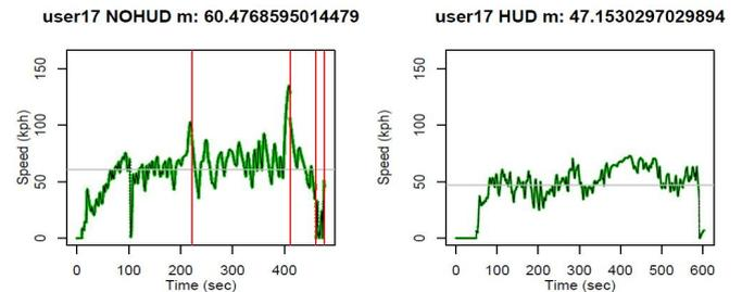
Figure 2: Typical user collisions and responses without and with the HUD
