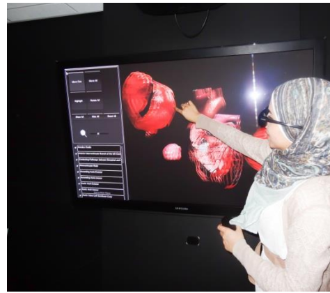
Fig. 6. Remote manipulation of 3D data in semi-immersive environment (3D TV). This Figure shows the researcher using the system in the Virtual Reality laboratory using the 3D TV and wearing active stereo 3D glasses (Glasgow Caledonian University/United Kingdom)
