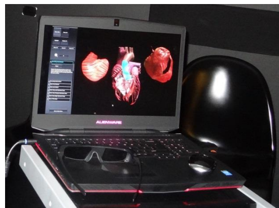
Fig. 7. Semi-immersive environment using common mouse/keyboard on a stereoscopic display. This Figure shows the VR Medical training System running using a powerful PC with a powerful graphic card and wearing active stereo 3D glasses to run the system. Virtual Reality laboratory (Glasgow Caledonian University/United Kingdom)
